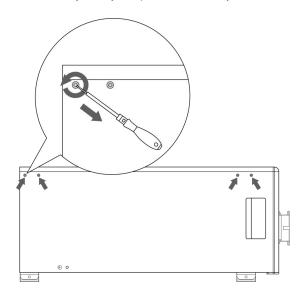
2) Secure 4 brackets to two sides of every battery with 8 bolts (M3\*10) mentioned in the step 1.
