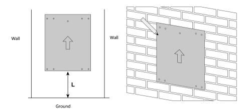
How to differ the floor-mounted installation from the wall-mounted installation mainly depends on the **clearance L** between the ground and the positioning cardboard.
