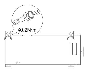
3) Stack the battery one by one and then secure them with 4 bolts (M4\*12). The number of stacked batteries can not exceed 6.
